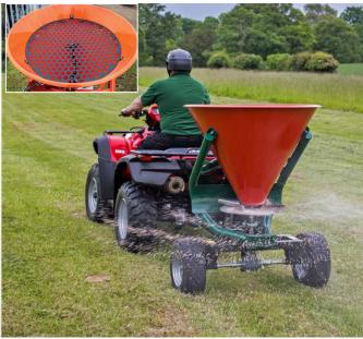
Paddocks, lawns and driveways are all taken care of with the trailed spreader range. With a choice of two sizes of hopper capacity, these spreaders are perfect for use behind ATV's and road vehicles. An agitator in the hopper improves material flow while the optional winter kit is invaluable for accurate spreading of free-flowing granular salt.
